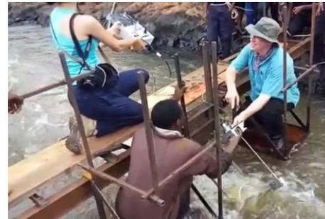
In the image above: RPP generating electricity in the Rupingazi River – suspended from a bridge/working platform made and installed by Don Bosco Technical College, Embu.
